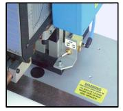
Optional Air Pressure On-Off Switch Can Control Air Supply to Both Tab Feeder/Cutter and Welder
